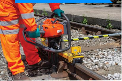
The NEW Master 35<sup>®</sup> Impact Wrench is powered by a New Generation low emission 63.4 c.c. Engine complying with EUR5 and EPA3 Standards which is a significant step towards de-carbonisation.
